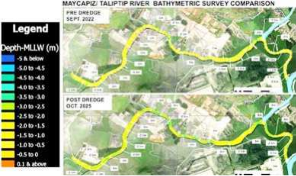
Bathymetric survey shows the Maycapiz-Talipit River prior to SMC's cleanup efforts in September 2022 (top) and its current state (bottom), highlighting improved carrying capacity and flow. From shallow depths of mostly .5 to 1.5 meters, the river is now 3-4 meters deep, allowing for improved flood mitigation and more efficient drainage out to Manila Bay.
